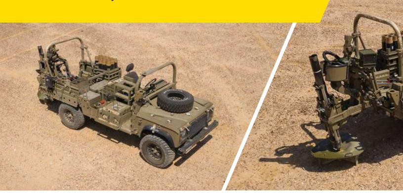
A fully autonomous, computerized, mounted mortar system with the dimensions and weight of a small carrier vehicle, the SLING is adaptable to a wide range of high mobility platforms. The rapidly deployed 120mm mortar system enables quick response and enhanced survivability, in and out of action within 30 - 60 - seconds, with shoot and scoot capabilities. Sling is easily operated by a 2 – 4 person crew.
